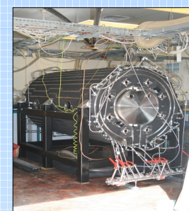
Fig. 5: The HIRAC chamber equipped with recently installed temperature control system.
