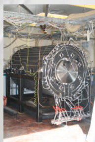
Fig. 8: Installation of the HIRAC temperature control system.
