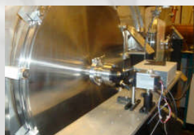
Fig. 4: Picture of the a mirror mounted on HIRAC.
