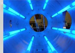
Fig. 2: Photolysis lamps.
